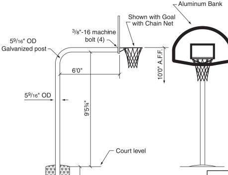
Specifications- 5065XY Outdoor Backstop—59/16" Gooseneck Post with 6' Extension
