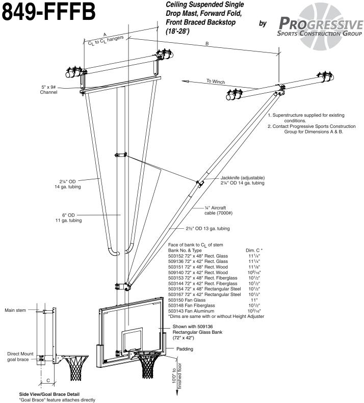
"Goal Brace" feature attaches directly behind goal mounting plate and directly to main stem of backstop, which eliminates strain on backboards.
